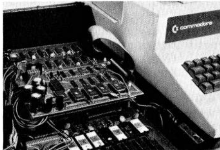
The Skyles MacroTea and Memory Boards hooked up to an original PET2001-8 (expanded to 32K). "A tremendous amount of stuff in unbelievably small space," says Skyles.
